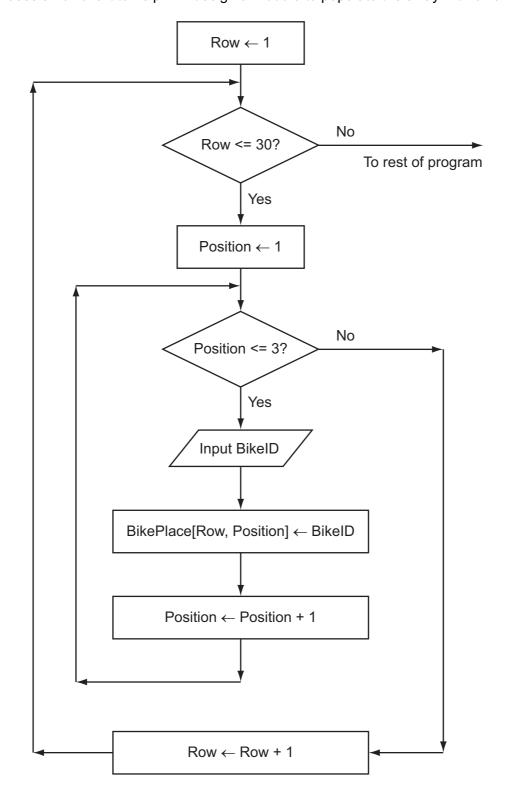
(a) Complete the trace table for the flowchart with the first five bike IDs. The values to be entered are BIKE34, BIKE56, BIKE70, BIKE51 and BIKE19.
