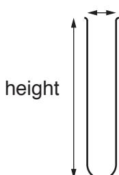
When small test-tubes are provided, it is expected that these are approximately 150 mm in height.
