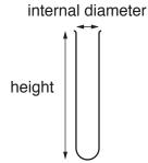
When small test-tubes are provided, it is expected that these are approximately 150 mm in height.
