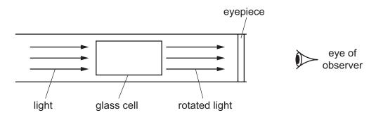
If a glass cell of length 10 cm is filled with a solution of sucrose of concentration  $1 \text{ g cm}^{-3}$  the measured angle of rotation is known as the specific rotation, [ $\alpha$ ].
