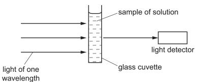
(a) (i) A chemist placed distilled water in the glass cuvette. This was then put into the spectrophotometer and a reading taken.
