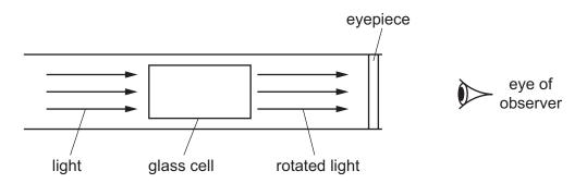
If a glass cell of length 10 cm is filled with a solution of sucrose of concentration  $1 \text{ g cm}^{-3}$  the measured angle of rotation is known as the specific rotation, [ $\alpha$ ].
