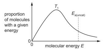
Which diagram correctly shows the new distribution and new activation energy,  $E_{a(cat)}$ , when the temperature is increased to  $T_2$ , and a catalyst is used that increases the rate of the reaction?
