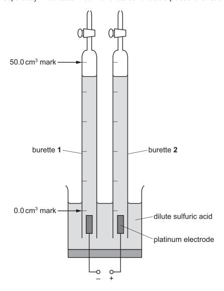
reaction at electrode in burette 1:  $2H^+(aq) + 2e^- \rightarrow H_2(g)$  reaction at electrode in burette 2:  $H_2O(I) \rightarrow \frac{1}{2}O_2(g) + 2H^+(aq) + 2e^-$
