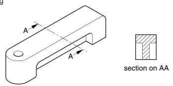
Runner for sliding doors Process: extrusion
