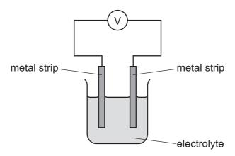
Which pair of metals produces the highest voltage?
