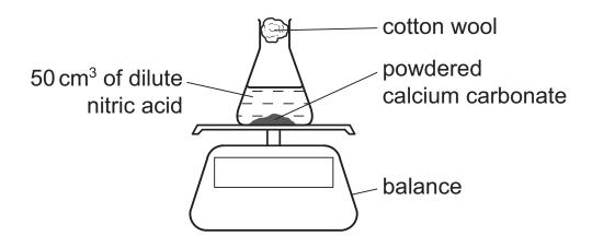
Excess powdered calcium carbonate was added to the nitric acid and the mass of the beaker and contents recorded. The time taken for the mass to decrease by 1 g was measured. The experiment was repeated at different temperatures.
