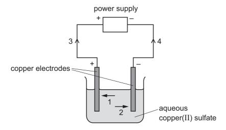
Which arrows indicate the movement of the copper ions in the electrolyte and of the electrons in the external circuit?
