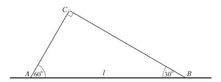
Two straight uniform ladders, AC and BC, have equal weights W. They stand in equilibrium with their feet, A and B, on rough horizontal ground and their tops freely hinged at C. Angle  $CAB = 60^{\circ}$ , angle  $CBA = 30^{\circ}$  and AB = l (see diagram). Find the vertical reactions at A and B.
