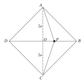
ABCD is a smooth square horizontal table with centre O and diagonals of length 4a. A particle P of mass m rests on the table and is connected to A and to C by two light elastic strings, each of natural length a and modulus of elasticity  $\lambda$  (see diagram). Show that, when P is displaced a short distance x from O towards B, the resultant force towards O is  $\frac{\lambda x}{a}$ , if  $\left(\frac{x}{a}\right)^2$  and higher powers of  $\frac{x}{a}$  are neglected. [5]
