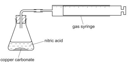
The volume of carbon dioxide produced was measured every minute for six minutes.
