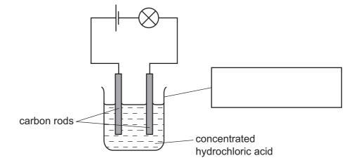
During the experiment, bubbles were observed at both carbon rods.
