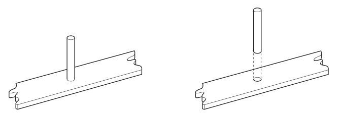
**C** drill and bend the acrylic frame and glue the acrylic rod to the acrylic frame.
