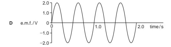
**37** A waveform is displayed on a cathode-ray oscilloscope. The length of three cycles of the waveform is 6 cm. The vertical gain and the time-base settings are shown on the diagram.
