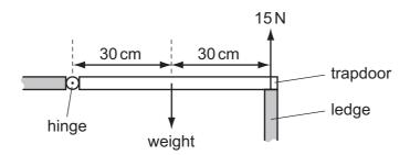
When the trapdoor is closed, the ledge exerts an upward force of 15 N on the trapdoor. The gravitational field strength is  $10\,\text{N/kg}$ .
