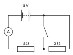
What is the reading on the ammeter when the switch is open, and the reading when it is closed?
