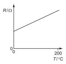
The resistance of the wire at  $0\,^{\circ}\text{C}$  is  $1.00\,\Omega$  and at  $100\,^{\circ}\text{C}$  is  $1.40\,\Omega$ .
