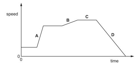
**4** An object falls from rest through the air and the air resistance on it increases. The object reaches terminal velocity.
