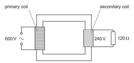
What is the power dissipated in the resistor and the current in the primary coil?
