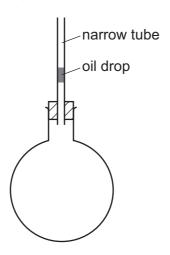
When the flask is heated the oil drop rises up the tube.
