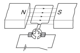
The switch is closed and the coil rotates.
