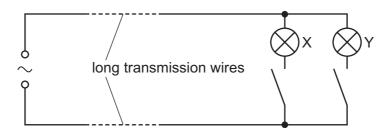
The identical lamps X and Y are connected to a low voltage a.c. power supply by high resistance transmission wires. Both lamps are switched on.
