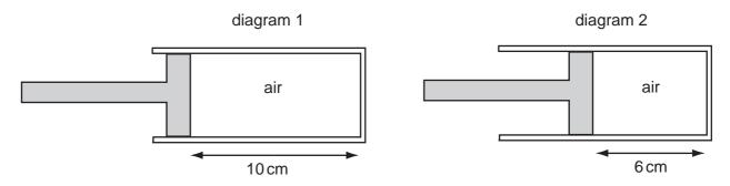
What is the pressure of the air in diagram 2?
