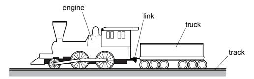
The link between the truck and the engine breaks. The driving force on the engine remains constant.
