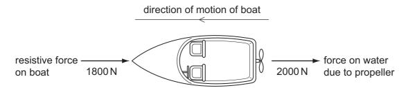
According to Newton's third law, what is the forward force on the propeller due to the water?
