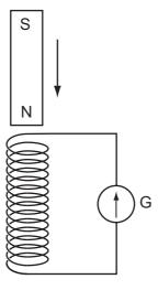
When a magnet is allowed to fall towards the coil, the galvanometer pointer gives a momentary deflection to the right of the zero position.
