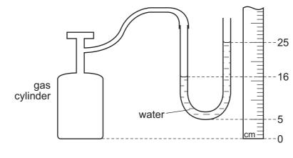
What is the pressure difference, in cm of water, shown by the manometer?
