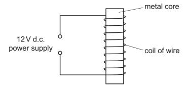
The core becomes a magnet when the current is switched on. It remains a magnet after the current is switched off.
