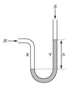
Side X is connected to a gas supply of pressure *R*. Side Y is open to the atmosphere at pressure *S*.
