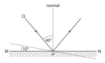
The mirror is rotated through  $10^{\circ}$ , as shown by the dashed line. The direction of the incident ray OP does not change.
