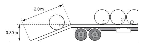
What is the work done on the barrel against gravity?
