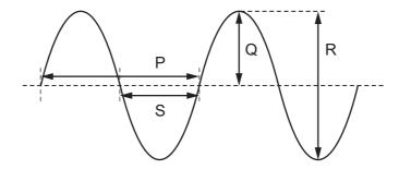
Which lengths represent the amplitude and the wavelength of the wave?
