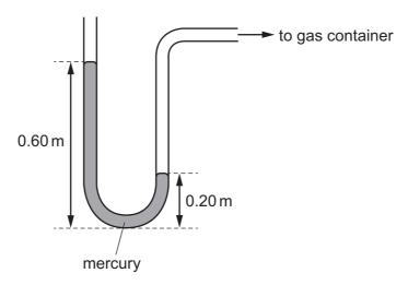
The density of mercury is  $14\,000\,\mathrm{kg/m^3}$ . The gravitational field strength g is  $10\,\mathrm{N/kg}$ .
