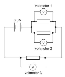
The reading on voltmeter 1 is 2.0 V.
