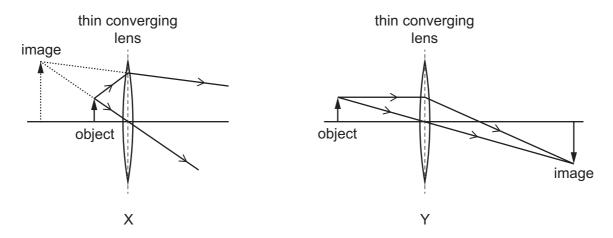
Which devices use a lens as shown in diagram X and in diagram Y?
