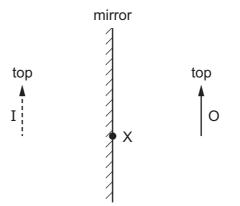
A ray from the top of the object is incident on the mirror at X.
