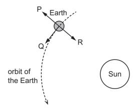
Which arrows show the direction of the acceleration of the Earth and the direction of the velocity of the Earth?
