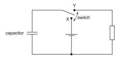
The switch can be moved between position X and position Y.
