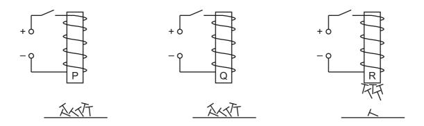
Which row identifies whether the core metals are ferrous or non-ferrous?
