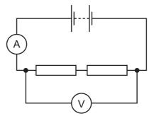
The voltmeter reading is 2.2V and the ammeter reading is 0.25A.
