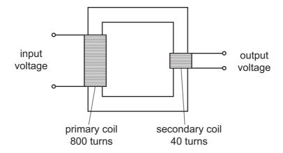
The input voltage is 240 V.
