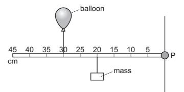
The balloon is filled with helium, a gas less dense than air, so that it applies an upward force on the rod.
