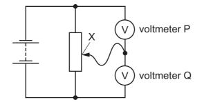
The sliding connection at point X is moved towards the top of the diagram.
