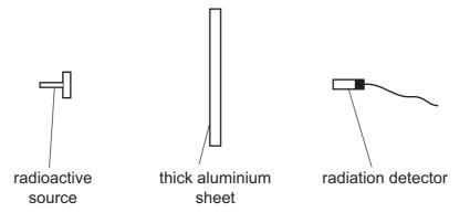
The radiation detector shows a reading greater than the background reading.
