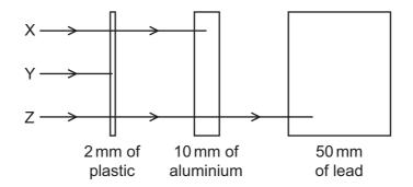
Which row in the table correctly identifies X, Y and Z?
