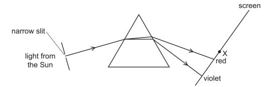
A thermometer placed at X shows a large temperature increase.
