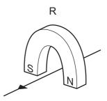
current direction reversed and magnet turned around
