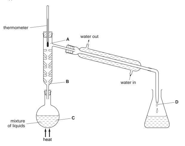
When the thermometer first shows a steady reading, at which point **A**, **B**, **C**, or **D** will there be the highest proportion of the liquid with the higher boiling point?
