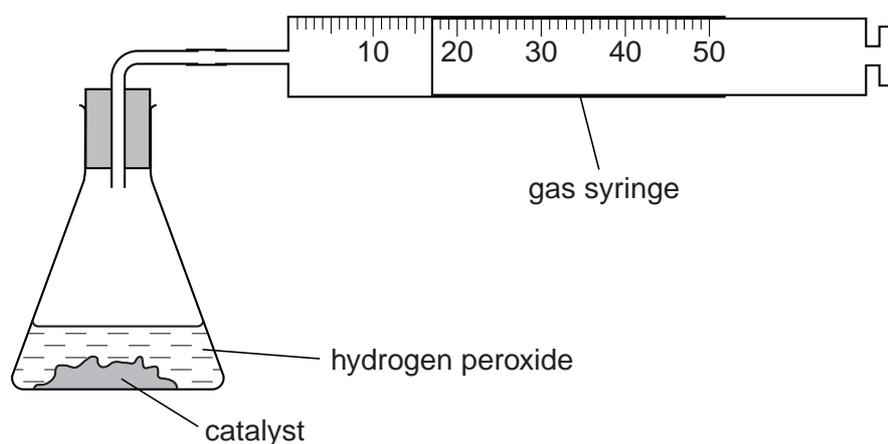
The student carried out two experiments using the same volume of hydrogen peroxide but with the same mass of a different catalyst in each experiment.
