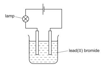
Why does the lamp light up only when the lead(II) bromide is melted?
