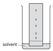
The solvent front is allowed to reach the top of the paper before the chemist removes the paper from the solvent.
