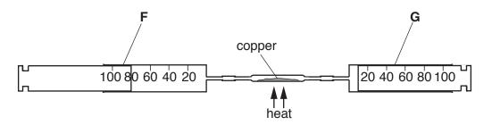
At the start of the experiment there is  $90 \text{ cm}^3$  of air in the apparatus. The air is passed backwards and forwards between gas syringes **F** and **G** over the heated copper. This is repeated until the volume stops decreasing. The gas is allowed to cool to room temperature and the final volume is measured.
