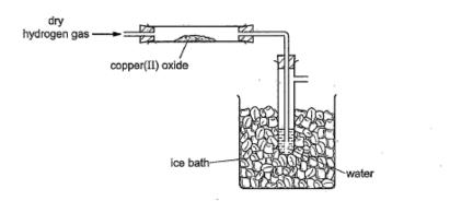
The hydrogen was passed over the hot copper(II) oxide until the reaction was complete.
