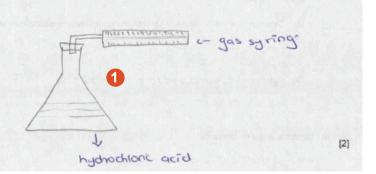
The gas syringe is labelled and there are graduation marks. There are no gaps in the apparatus. Both marks were given, although the drawing could have been improved. Both marks were given although the drawing could have been improved by not showing the stopper cutting across the delivery tube.
