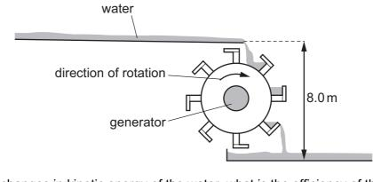
Ignoring any changes in kinetic energy of the water, what is the efficiency of the system?
