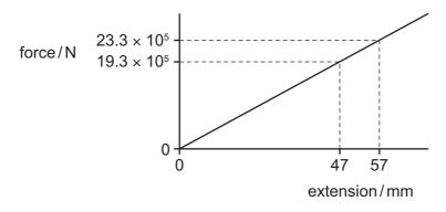
What is the increase in strain energy in the cable when the lorry is crossing the bridge?
