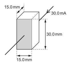
The electrical meters used are accurate to  $\pm$  0.1 mA and  $\pm$  0.1 V. The dimensions of the block are accurate to  $\pm$  0.2 mm.
