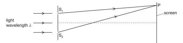
The *n*th **dark** fringe from the central bright fringe is observed at point P on the screen.
