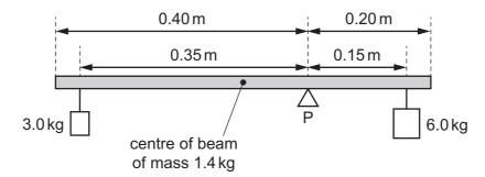
What is the torque that must be applied to the beam in order to maintain it in equilibrium?
