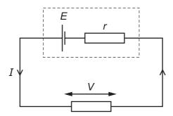
The current in the circuit is I and the potential difference (p.d.) across the external resistor is V.
