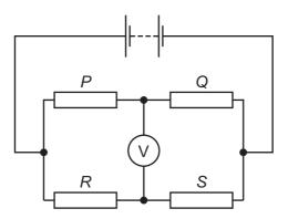
The voltmeter reading is zero.
