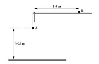
Particles A and B have masses 0.32 kg and 0.48 kg respectively. The particles are attached to the ends of a light inextensible string which passes over a small smooth pulley fixed at the edge of a smooth horizontal table. Particle B is held at rest on the table at a distance of 1.4 m from the pulley. A hangs vertically below the pulley at a height of 0.98 m above the floor (see diagram). A, B, the string and the pulley are all in the same vertical plane. B is released and A moves downwards.
