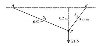
A particle *P* of weight 21 N is attached to one end of each of two light inextensible strings,  $S_1$  and  $S_2$ , of lengths 0.52 m and 0.25 m respectively. The other end of  $S_1$  is attached to a fixed point *A*, and the other end of  $S_2$  is attached to a fixed point *B* at the same horizontal level as *A*. The particle *P* hangs in equilibrium at a point 0.2 m below the level of *AB* with both strings taut (see diagram). Find the tension in  $S_1$  and the tension in  $S_2$ . [6]
